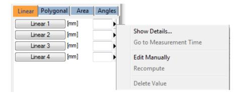
By clicking on the little arrow and then on *Show Details*, a window will be displayed in which all the samples taken for that item are shown together with the average and the standard deviation.
